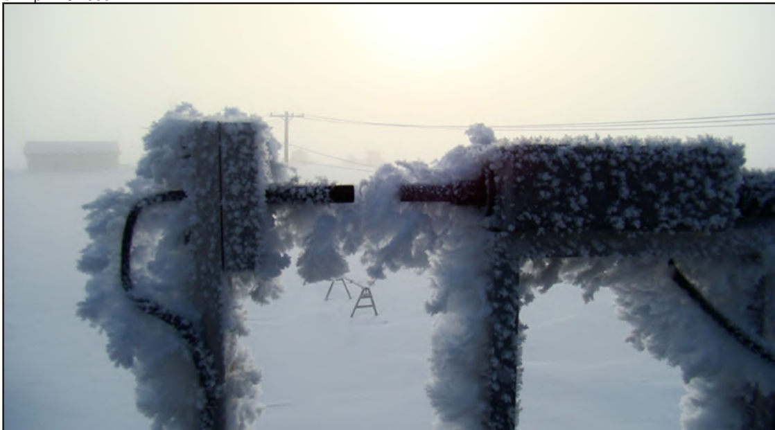
Figure 8: Frost formation on ice particle counter sensor which occurred during the FRAM ice fog project in Barrow, AL, on April 16 2008.
